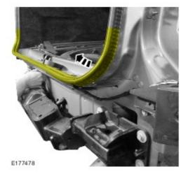
Reposition the tailgate aperture seal.
