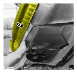
Install the tailgate aperture seal.
