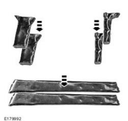
Stick two equal seal pads together to make the seal pads double the thickness.
