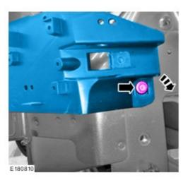
Remove the rear bumper cover corner bracket from the rear panel of the vehicle.
