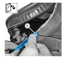
Locate and install the seal pad against the panel edge, as shown in the illustration.
