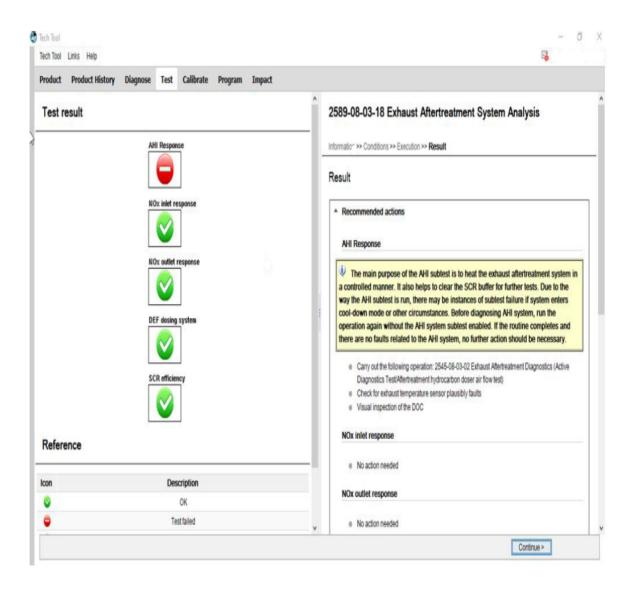
The "Not tested" response shown under the AHI Response section in the screenshot below is the result of unchecking the AHI subtest.
