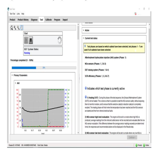
The screenshot below shows the current recommended actions for the scenario when criteria are met for the Heating EATS phase, except NOx outlet sensor came online just after the timeout period.
