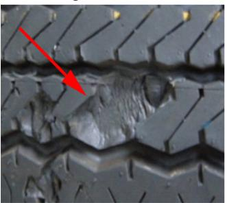
The condition shown in the above may be seen on new vehicles at the time of delivery to the dealer. The condition, known as "tire chunking" is not transportation damage, but damage from Dynamic Vehicle Testing (DVT) at the assembly plant.
