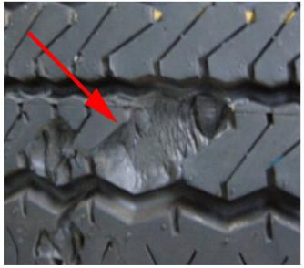
The condition shown in the above may be seen on new vehicles at the time of delivery to the dealer. The condition, known as "tire chunking" is not transportation damage, but damage from Dynamic Vehicle Testing (DVT) at the assembly plant.
