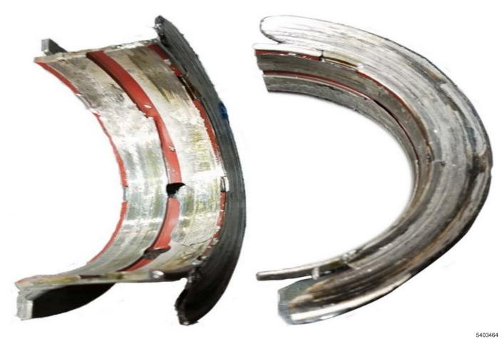
3. Inspect the thrust bearing for wear on one side and crankshaft on the corresponding mating surface. The graphic above shows an example of a damaged thrust bearing.
