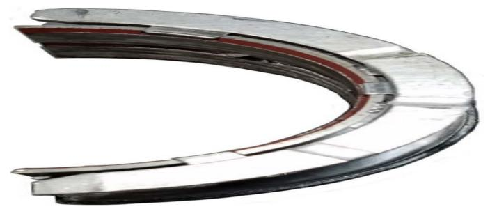
Example of a good thrust bearing face.
