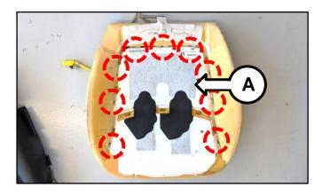
8. Using the SST 09880 4F000A, insert each clip through the retaining ODS sensor pad and crimp to the seat cushion rod to secure pad.
