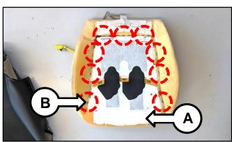
Using a heat gun, carefully apply heat to the front pad area shown to loosen the adhesive backing from the ODS sensor pad.
