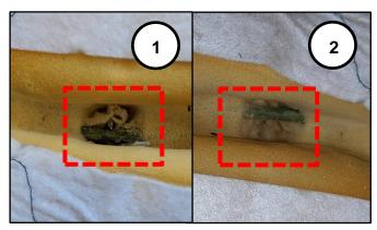
Lay the new ODS sensor pad (A) by aligning all of the nine (9) ODS sensor pad tabs to the seat cushion <u>and</u> route the coax cable down and in through the existing cushion cutaway shown below.
