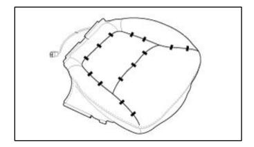
2. Using wire cutters, cut the nine (9) ODS retaining pad (A) clips (B).
