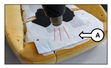
On the reverse side of the seat cushion, using a heat gun, apply heat to the ODS Module (C) to carefully remove it from the seat cushion.
