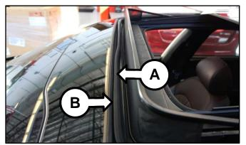
Partially remove the affected area of weather strip and clean the contact surface between the strip and sunroof frame using alcohol or a general purpose adhesive cleaner.
