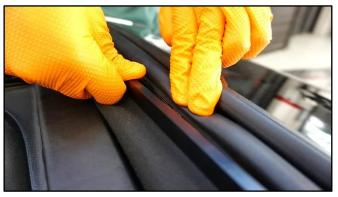
5. After ensuring that the adhesive has cured, open and close the sunroof several times to confirm proper installation of the weather strip.
