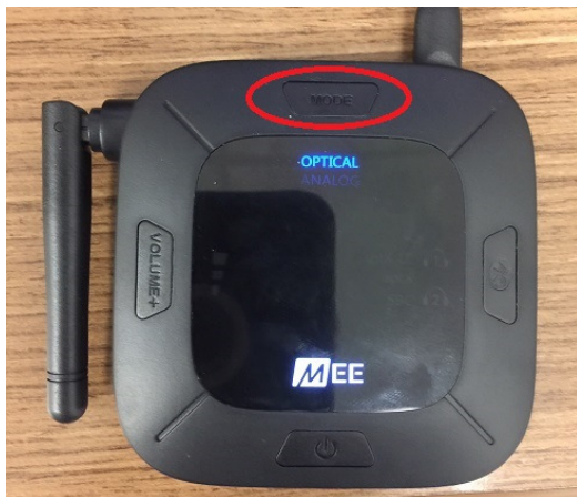
Figure 3: Proper audio mode for the Connect Hub, with OPTICAL lit up in blue and the Mode button shown.
