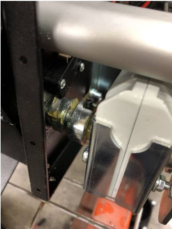
Pictured above is a shear pin that is broken and needs to be replaced.
