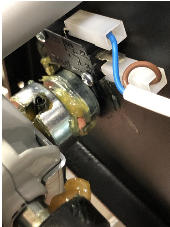
Pictured above is a shear pin that is broken and needs to be replaced.
