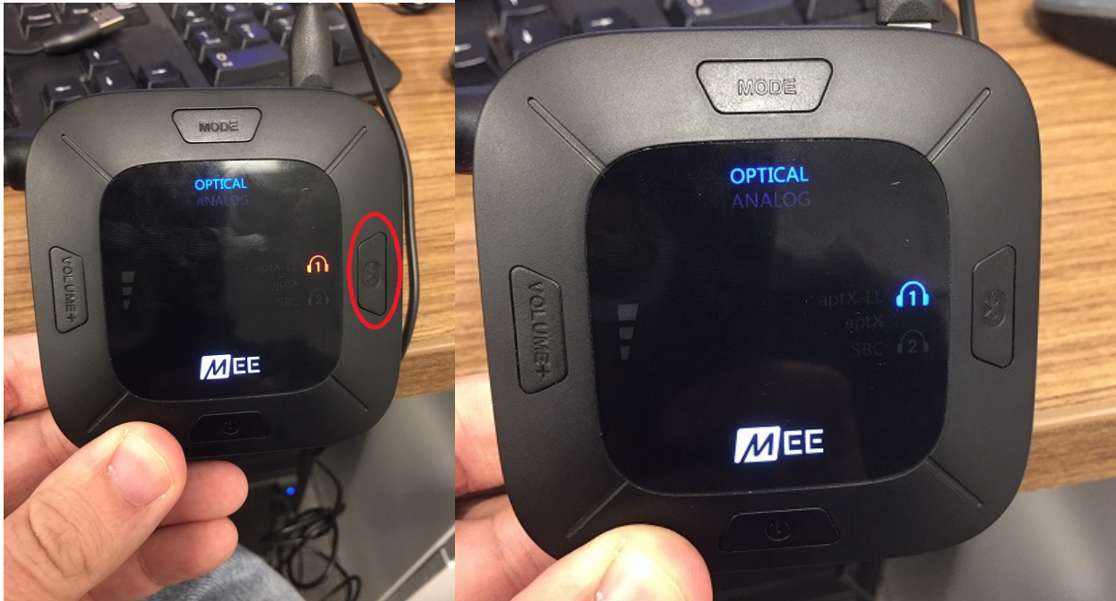
Figure 1a/b: Connect Hub in pairing mode, with the headphone icon flashing between red and blue and location of pairing button shown.
