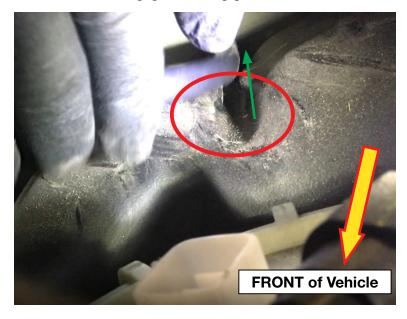
Using the illustrations and photos below as a guide, thoroughly clean the areas where the **Size A** and **Size B** EPT foam pieces will be applied using isopropyl alcohol on a clean shop cloth and allow to completely dry. Peel the backing and apply the two **Size A** foam pieces.
