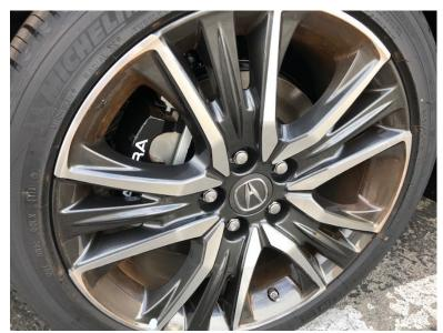
What you're seeing is just a buildup of rust on the brake discs from salt air during overseas transit. To remove that rust, just hose it off with water.
