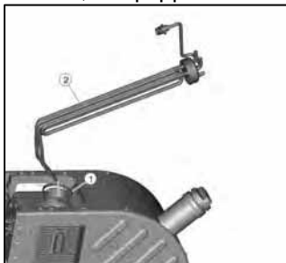
1. Level Sensor 2. Clamp
