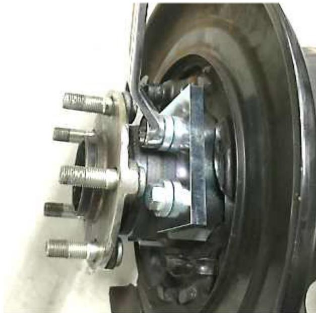
**NOTE:** Tighten the bolts in a crossing pattern to evenly apply axial force. If force is unevenly applied, the hub unit may stick in the housing and become extremely difficult to remove.
