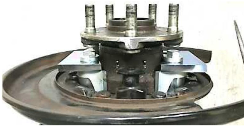
6. Remove the hub unit by tightening the bolts using a 14 mm box-end wrench in a crossing pattern as shown below.
