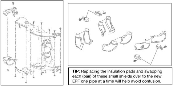
• Before applying any of the new insulation pads, wipe the inside and outside of the shields clean of any residual oil / penetrant used with a mild solvent on a clean shop cloth. Use caution to not remove the position markings for the replacement insulation pads.
