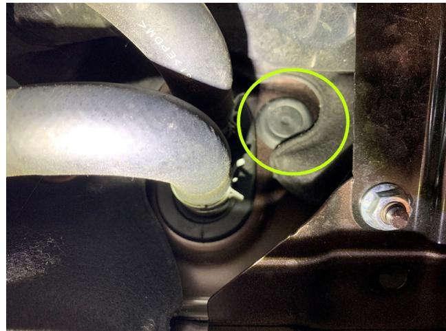
Remember to check the upper part of the cowl under the windshield. These plugs are smaller and can easily be overlooked. There are four located on this model and examples are found below.
