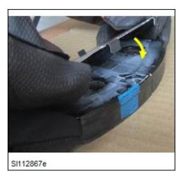
7. Remove the shim and confirm the grease has been applied evenly (as shown below).
