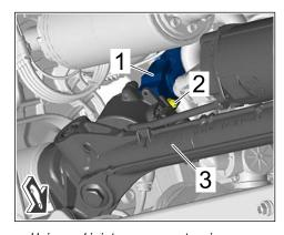
Universal joint on power-steering gear
