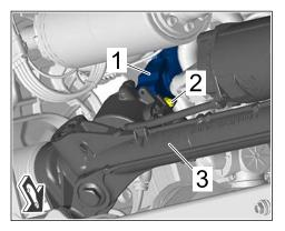
Universal joint on power-steering gear
