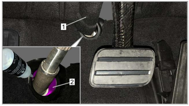
Steering column sealing bellows
