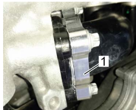
Installing water tube retaining bar
