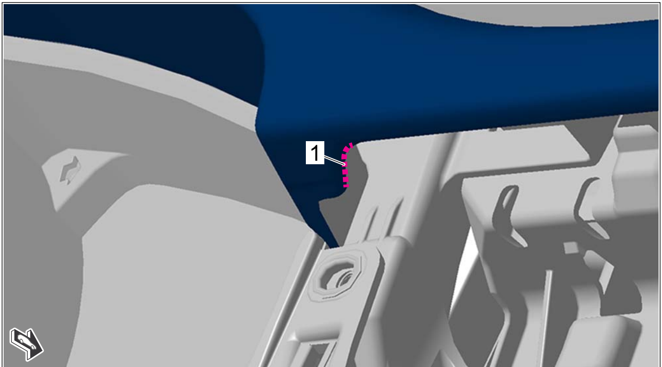
Reworking the top left corner of the dashboard
