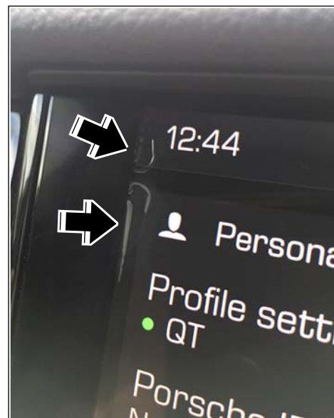
Air bubbles in the PCM display (example)
