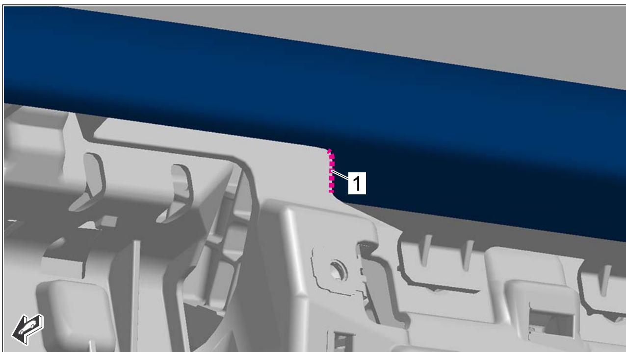
Reworking the top right corner of the dashboard
