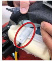
**Step7- CAREFULLY** peel the padding back to expose the tail and connections. Be advised, the adhesive used has a very strong grip. **CAREFULLY** peel the padding in a direction parallel to the tail and discard. A new piece of padding is included in the new replacement harness kit.
