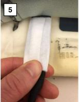
**Step11-** Use a scissor to cut the harness label from the original (removed) wiring harness.
