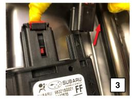
**Step6-** From the rear of the cushion (a cotter pin extractor works well), **CAREFULLY** release the plastic seat cover trim retainers as shown below and pull the back of the cover up as needed to access the harness to ODS sensor mat connection point (tail) circled below. The tail is covered in a self-adhesive fabric padding.
