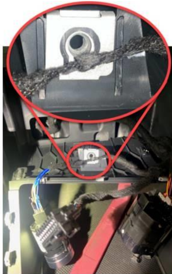
Figure 1. Wiring harness pinched at the mounting point.
