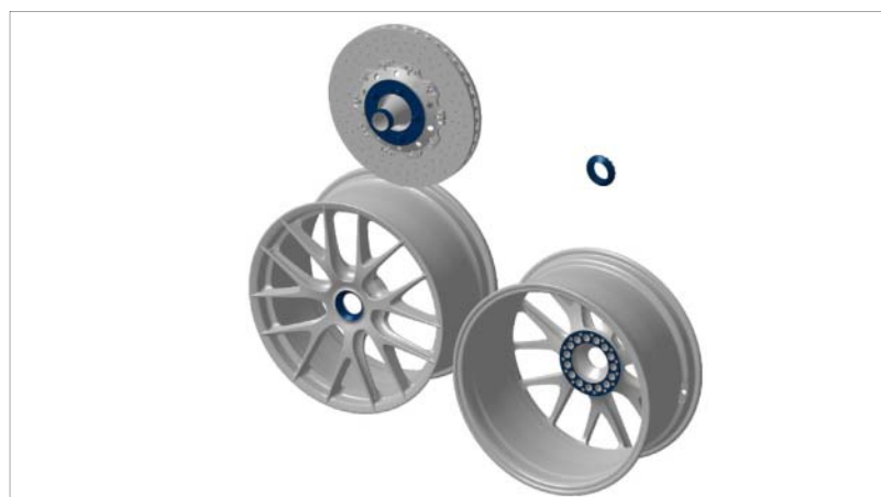
Cleaning contact surfaces of rim/brake disc
