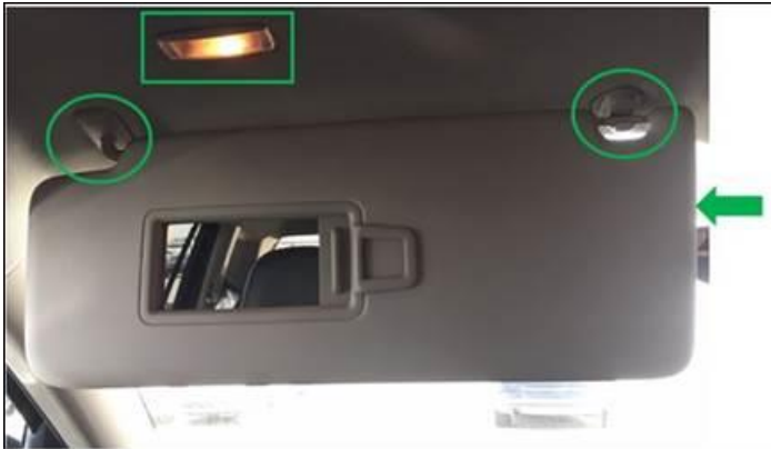
Figure 2. Correct – Sun visor in the correct position for vanity light operation.
