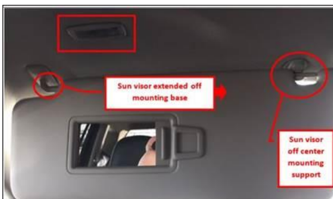
Figure 1. Incorrect – Sun visor extended away from the mounting base, vanity light inoperative
