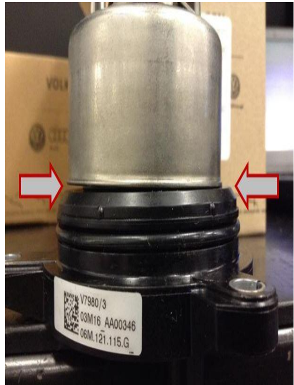
Figure 1. Gap between chamber and seal.
