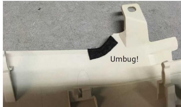
Figure 4. Apply the felt tape around the edge of the trim as shown.
