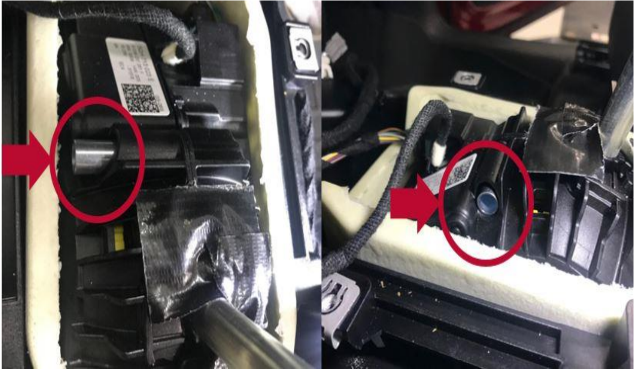
Figure 5. Installing the spacer sleeve.
