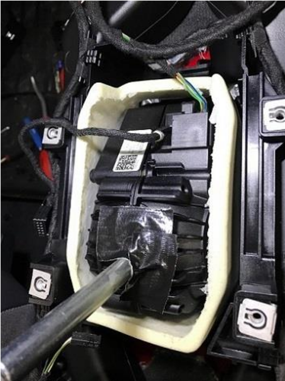
Figure 3. Tape covered shift gate.
