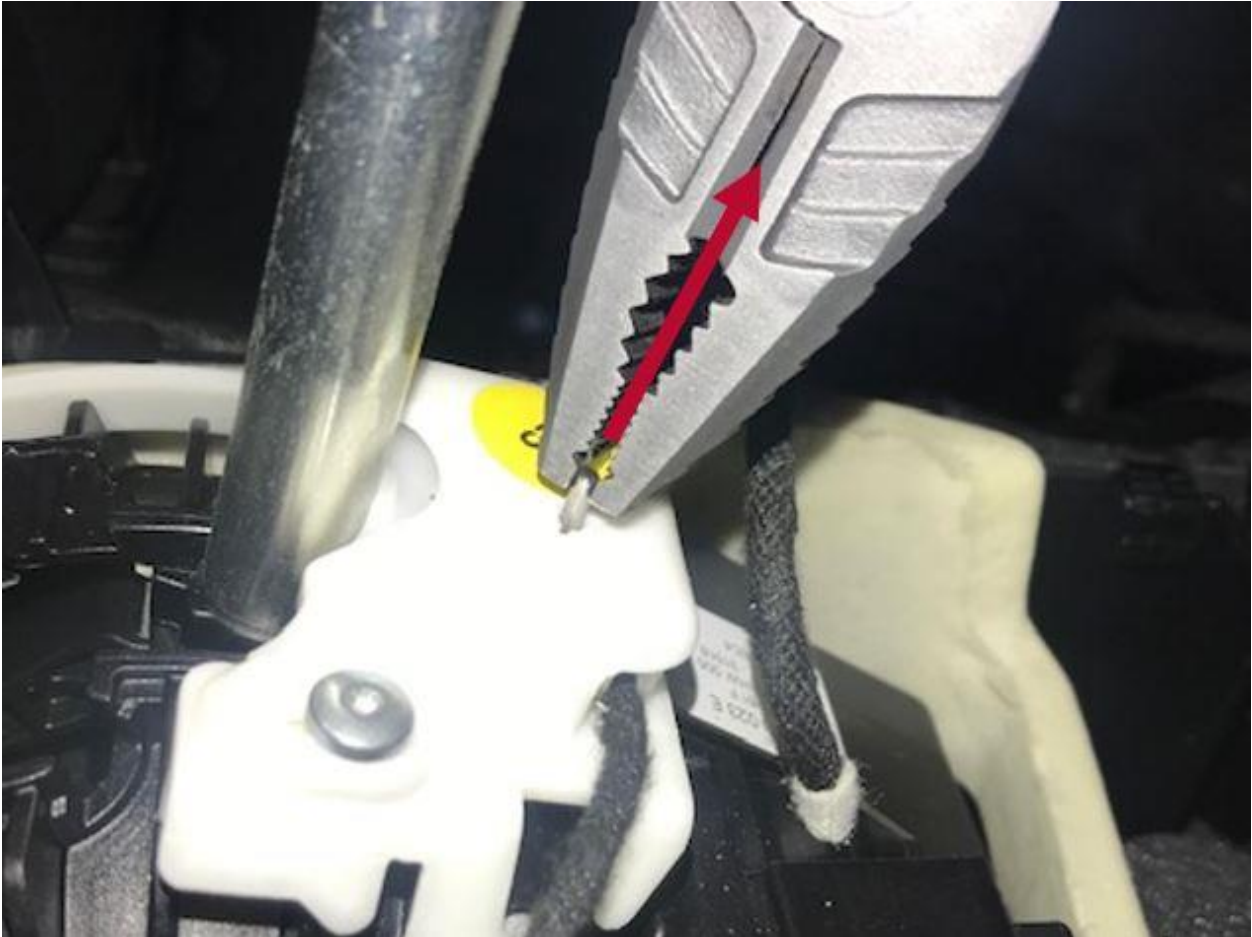
Figure 11. Removing lock pin from the microswitch module.
