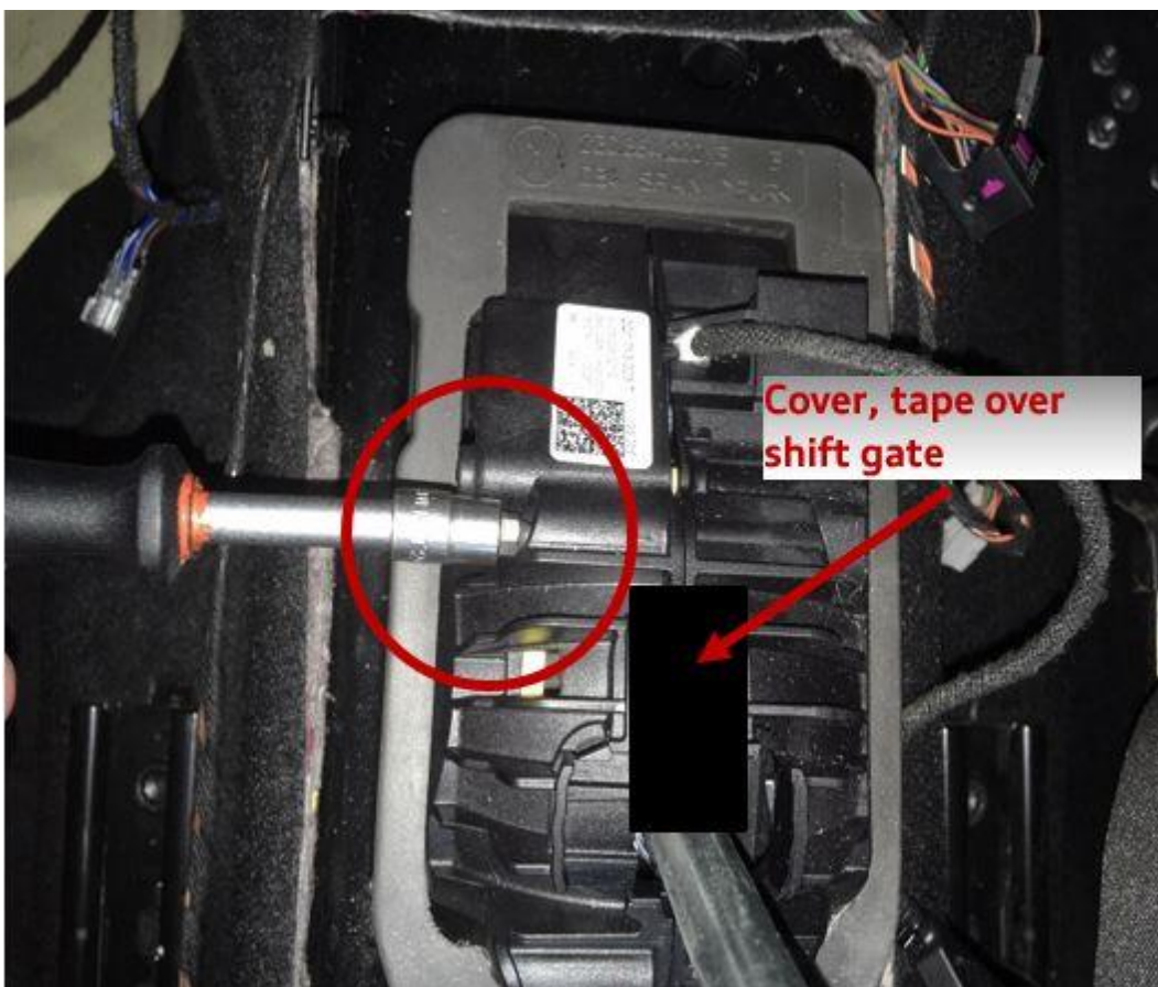
Figure 4. Removing T-20 screw.
