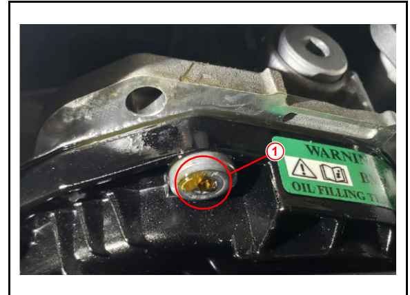
Figure 2. Oil Leak From Transmission Oil Pan
