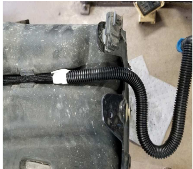
Original design fuel feed line at tank
