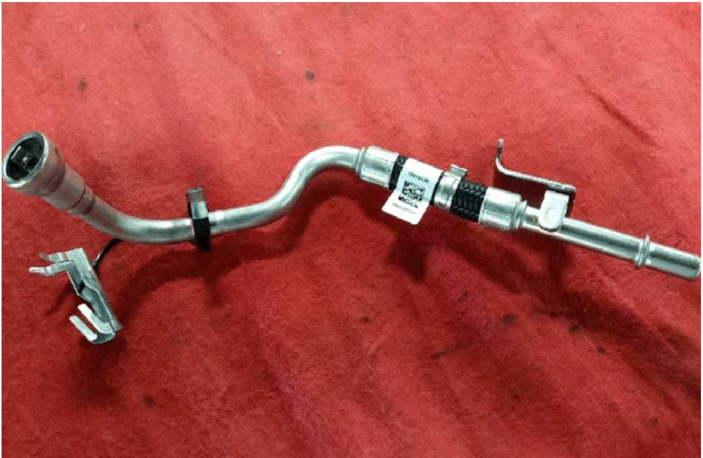
Low pressure fuel feed jumper pipe at engine
