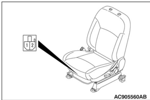
Connect the (+) terminal of the battery to the power seat connector terminal No.2 and the (-) terminal to terminal No.1, and check that the power seat works normally.
