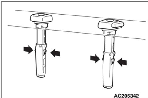
Peel off the front seatback cover and pad to access the headrest guides. Pull off the guides upwards while pushing the tabs (arrows) as shown.
