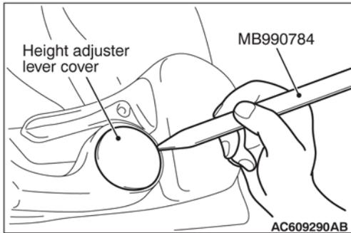
Use special tool MB990784 as shown to remove the height adjuster lever cap.
