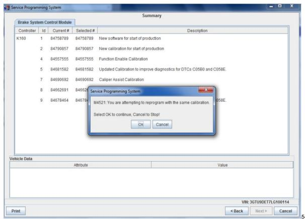
Important: If the Same Calibration/Software Warning is noted on the SPS screen, select OK and follow screen instructions. After a successful programming event, the WCC is located in the Service Programming System dialogue box of the SPS Summary screen. No further action is required. Refer to the Warranty section of the bulletin.
