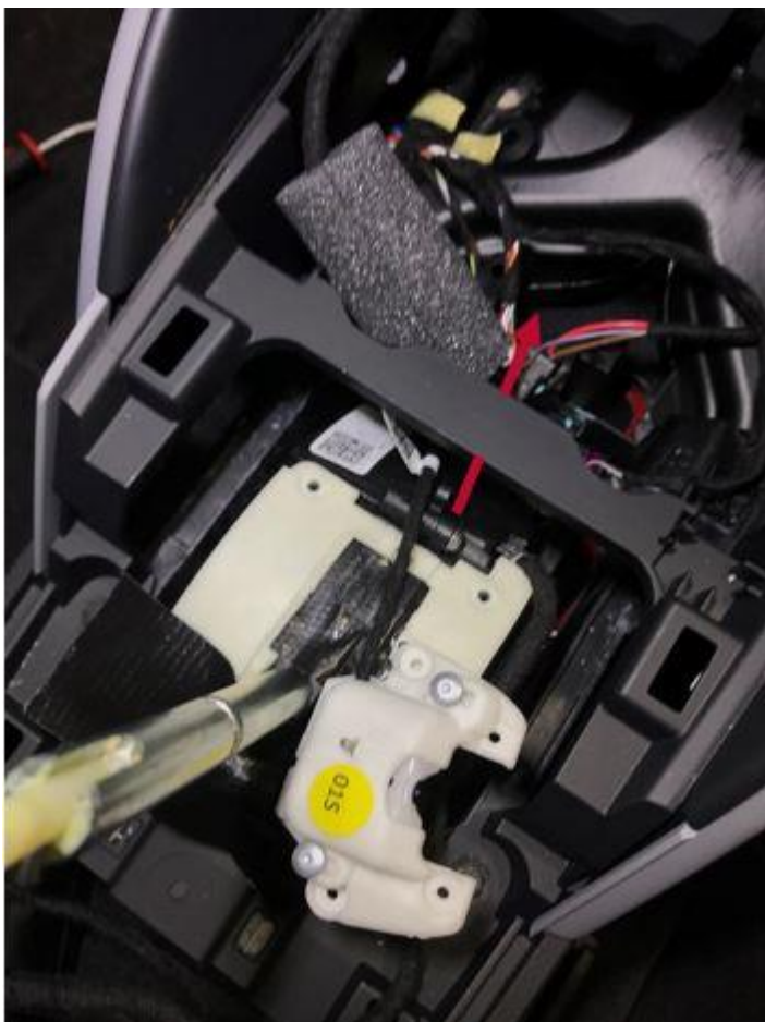
Figure 8. Wiring harness run under the crosspiece.
