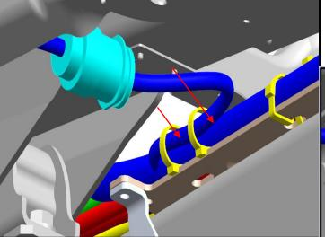
Reinstall the 87L bracket that now encases both the chassis harness and the air line bundle. Add one more tie strap as noted below
