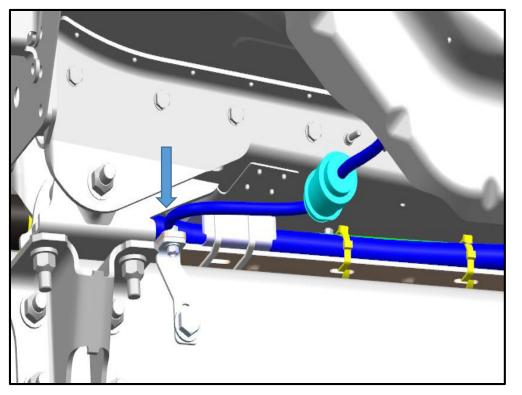
Follow the next three steps to remove the 87L content pneumatic bracket
