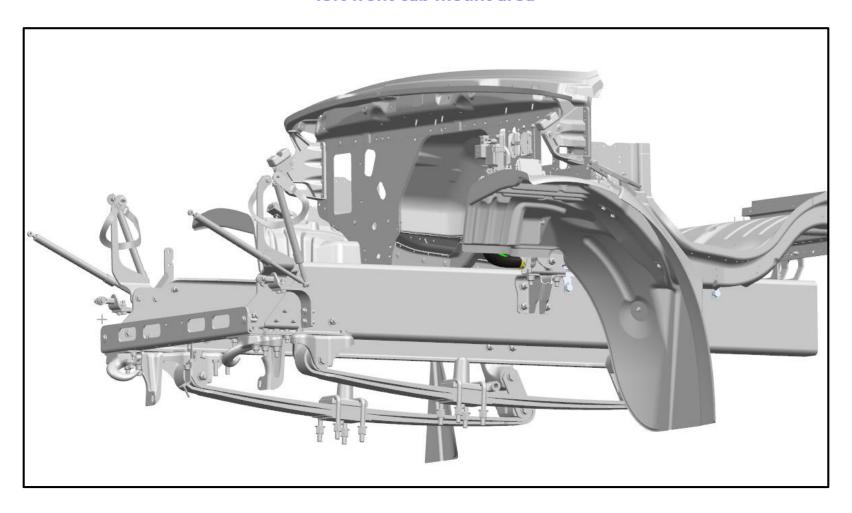
Remove fasteners to access 87L content pneumatic line bracket
