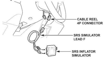
12. Connect the terminals of SRS simulator lead F to the SRS inflator simulator (2  $\Omega$  connectors), then connect SRS simulator lead F to the cable reel 4P connector as shown.
