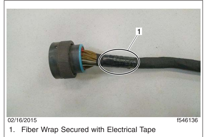
Fig. 15, Fiber Wrap Secured with Electrical Tape
