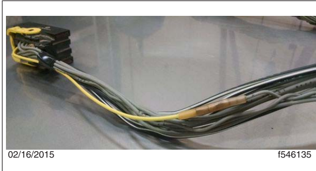
Fig. 5, Splicing the Wires
