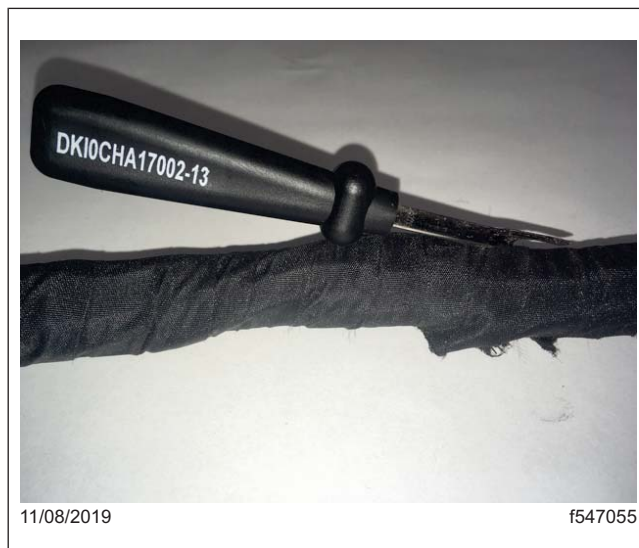
Fig. 10, Cutting the Fiber Using the Blunt End of the Seam Cutter
