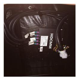
First do a hard reset on the HDCMM by pulling the power harness for 10 seconds, when troubleshooting any issue.
