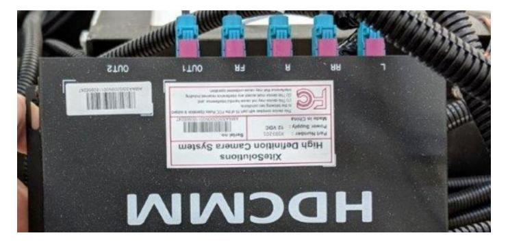
Each camera is the same and can be swapped around on the outside of the coach. The HDCMM determines which view is which. Be sure to install a replacement camera in the exact same location as the factory installed camera. This will insure the 360 image looks correct when done.
