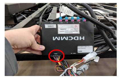
If no image is present from the HDCMM, on screen will be "No Video Detected". If after a hard reset the screen still shows "No Video Detected", **bypass the installed cable between "Out 1" and the Core with a tester cable.** This confirms whether or not the installed cable is damaged.
