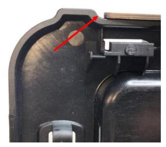
(arrow) using a file. A feeler gauge can be used (shown lying flat along top edge) to assist with measuring.
