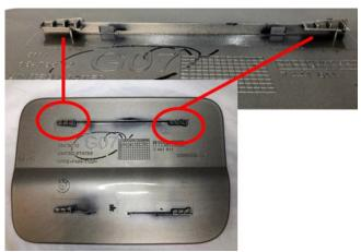
7. Apply a 5 mm section of butyl inside each locking tab of the filler door, in the area shown to the left.
