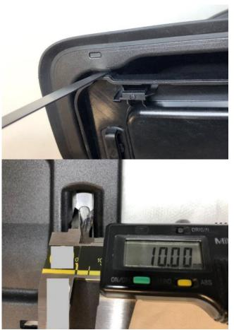
4. Close the filler flap and measure the distance between the upper tab and the filler door assembly. The gap must be at least 0.1 mm.
