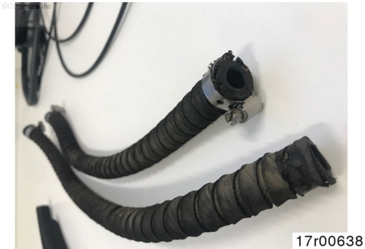
Figure 2, Old LP Fuel Hoses that are Susceptible to Cracking
