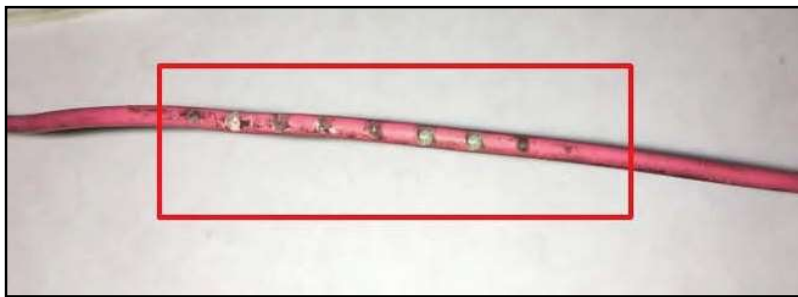
Figure 9 - Wire Conductor Copper Strands Visible
