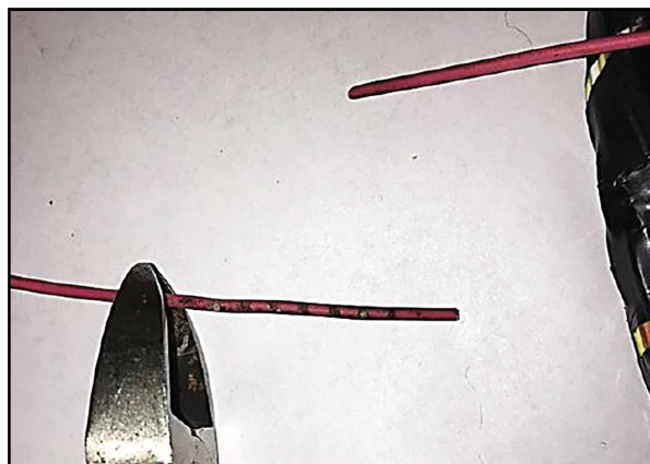
Figure 10 - Cut Wire Damaged Section
