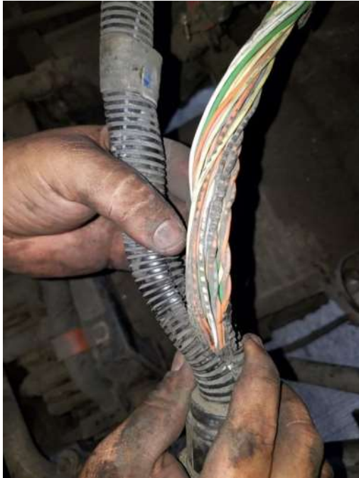
Figure 4 - Chafed Wires and Chafed Convoluted Tubing
