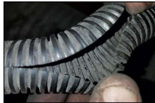
Figure 4 - Chafed Wires and Chafed Convoluted Tubing
