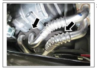
c. Reinstall the stud bolt using an E8 Torx socket.Torque: 10.0 N·m (102 kgf·cm, 84 in.lbs)
