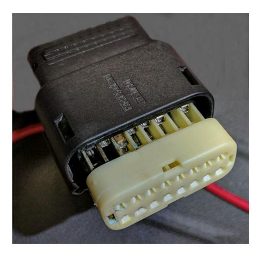
If water intrusion or corrosion is found replace all affected terminals on the body side with terminated leads and replace the rear fascia wiring harness.
