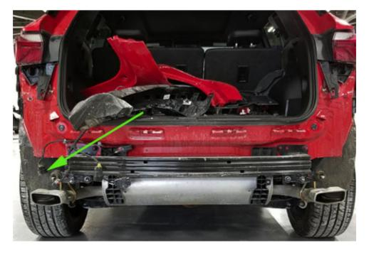
If no obvious terminal concerns are found it may be necessary to remove the TPA to be able to view inside the connector for moisture.
