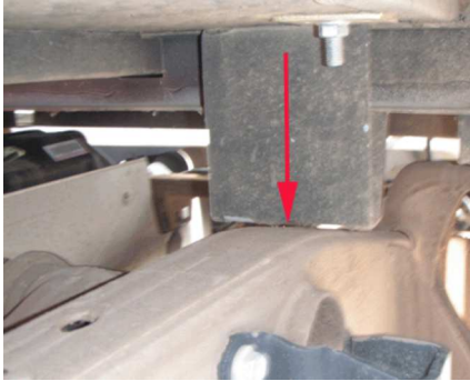
Example of support bracket not carrying any load of the body.
