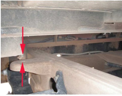
Example of available body mounting locations not used by the upfitter under the service body.
