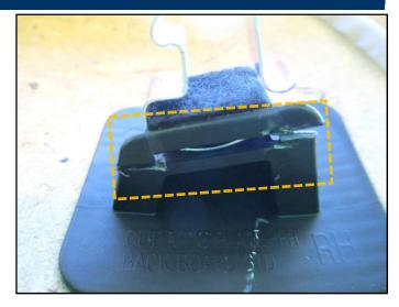
5. Remove the broken base clip, and remove excess plastic to ensure base (D) is flat.
