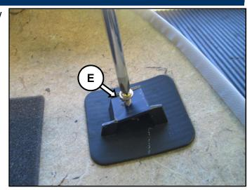
7. Assemble the screw (E) into the supplied new clip (F) and fully tighten to base.
