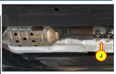
9. Reuse the rear flange gasket and install the new replacement center muffler (I) to the clamp (J), then temporarily hand tighten the flange nuts.
