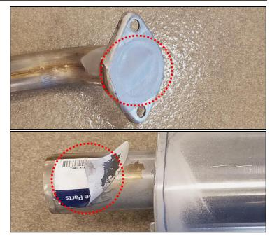
7. Reuse the front flange gasket and install the catalyst (F), then temporarily hand tighten the flange nuts.
