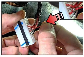
9. Push down on the secondary locking tab of the junction block to lock wires.
