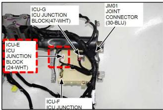
7. Using a pick tool, pull up on the secondary locking tab to unlock the white junction block wire Pins. Note: Two (2) pull inserts shown.
