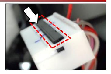
Secure the "red" wire to the junction block wire harness by using insulation adhesive tape if available. Electrical tape and/or zip-ties may also be used.
