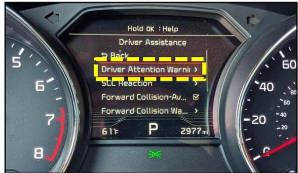
10. Select the desired Driver Attention Warning sensitivity level (Off, Normal or High), press 'OK' button to set. (Example below was set to Normal Sensitivity)
