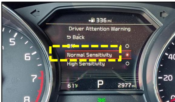
11. Scroll to **Back**, and press the **OK** button to exit. Press the **MENU** key to exit the main menu. The DAW setting is now complete.
