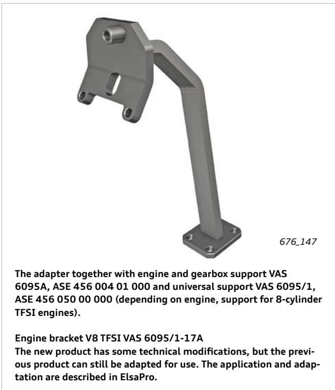
Engine bracket V8 TFSI VAS 6095/1-17
