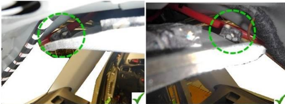
Figures 6 and 7, Rear drain hoses routed behind foam blocks on headliner.
