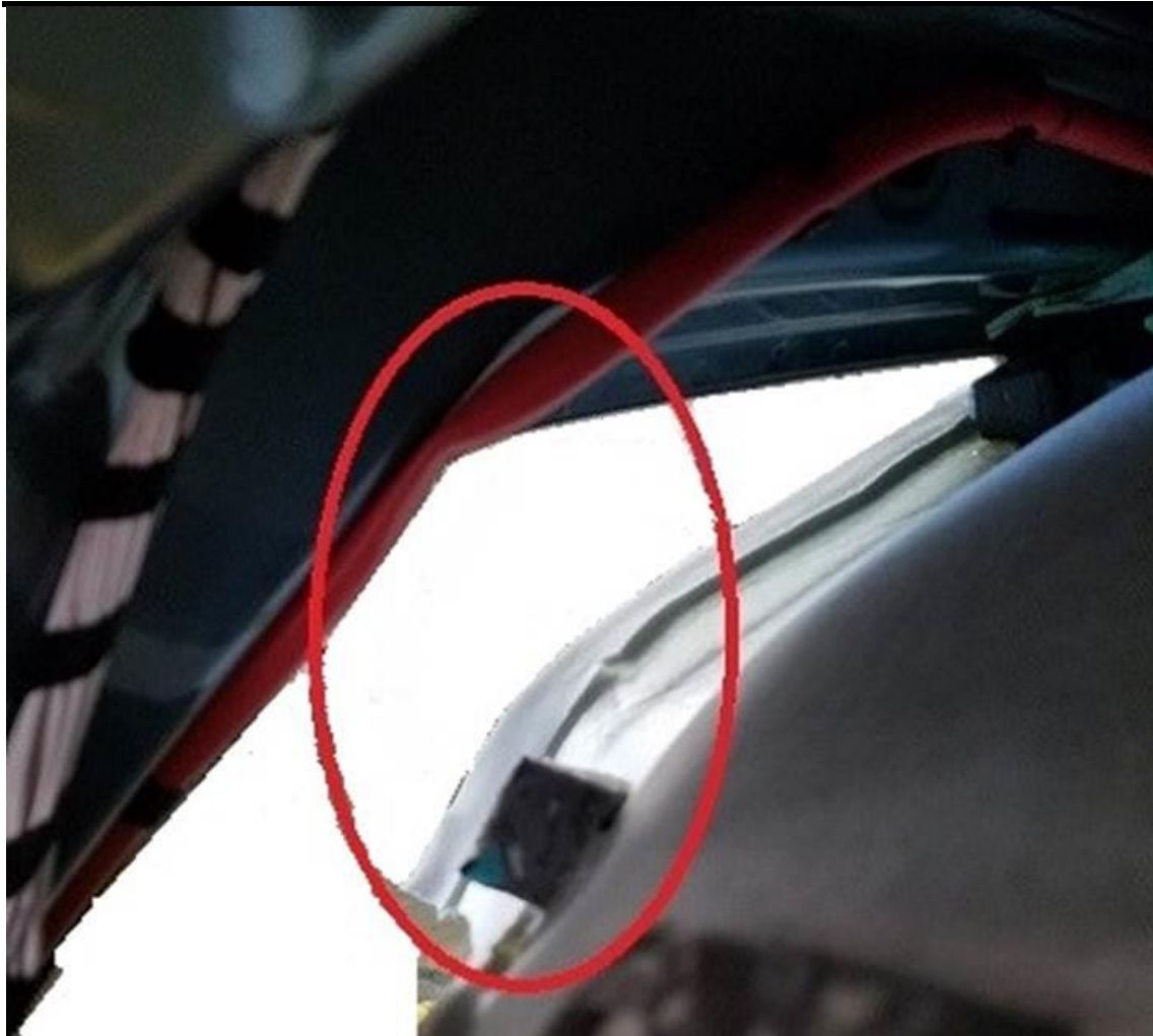
Figure 1: Sunroof drain pinched by foam block on headliner
