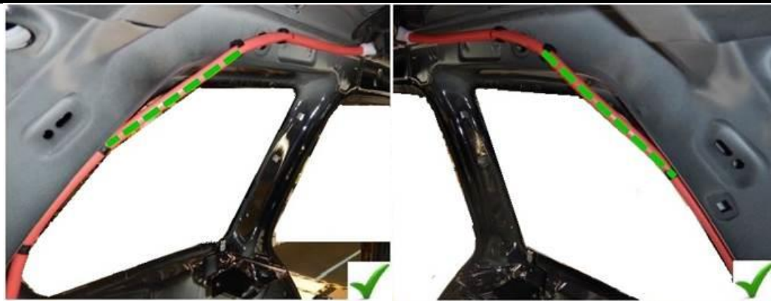
Figures 4 and 5: Correct routing of left and right rear drain hoses with no slack between the 2 nd and 3 rd mounting clips.
