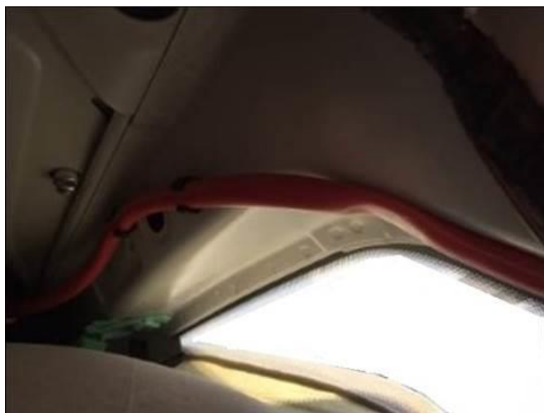
Figure 3: Impression on rear sunroof drain from contact with headliner foam block.
