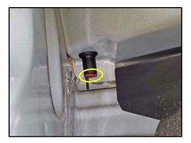
Remove flaps from left front and right front • sunroof drains.
