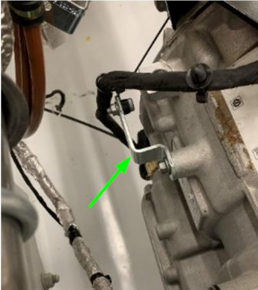
1. C) Dual Fuel Tanks configurations: Mount Fir tree 23-13482-003 below the fuel line bracket (The one used to mount the "Tee Valves").
