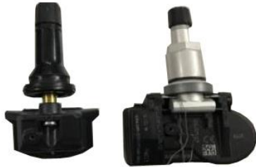
New Rubber Type Old Metal Type
