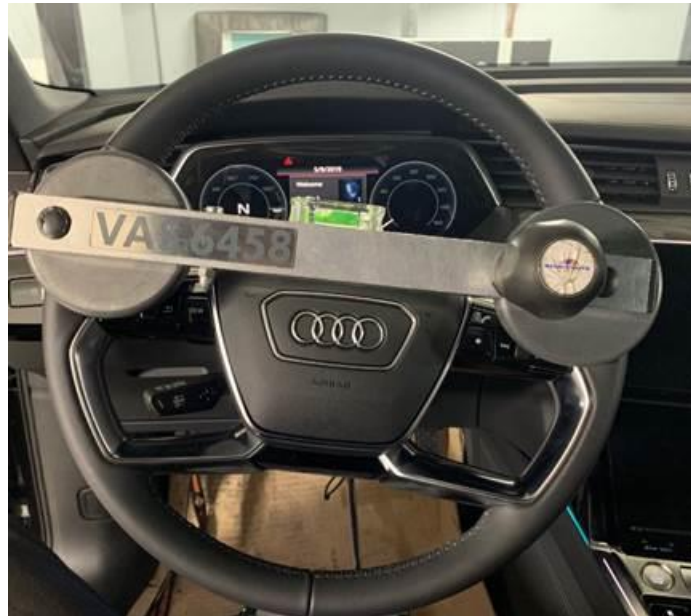
Figure 1. VAS 6458 installed with steering wheel off-center.
