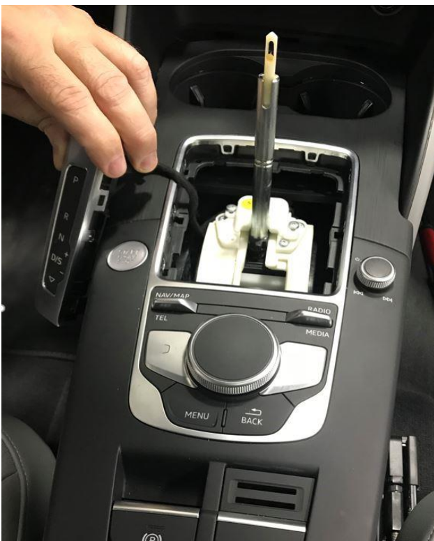
Figure 13. Console insert installed.
