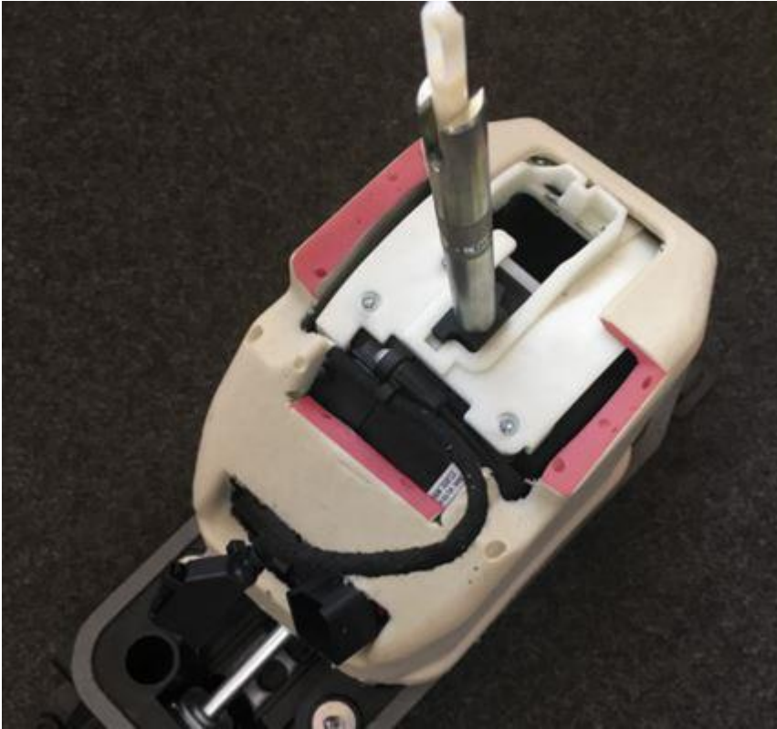
Figure 5. Example of modified insulation installed on a shifter housing.
